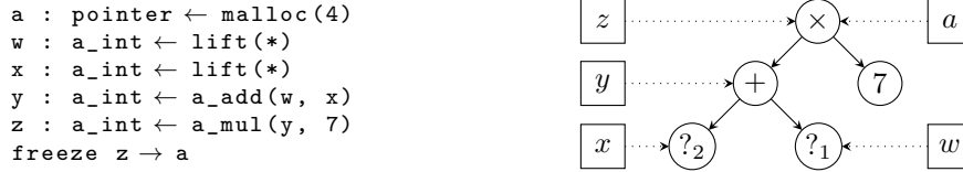
Fig. 5. Example of a formula tree as generated by the term domain. The boxes correspond to abstract variables, while the circles are the concrete representation of terms. Question marks denote unconstrained nullary symbols.
